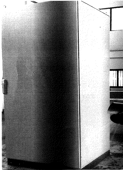
Photograph Number: CPRIBLREATD23T0378P04 During IP X4 – Water Test
